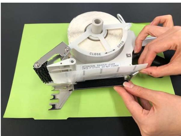
2. Place a label roll and put the Label Holder on it, then turn it clockwise to 'CLOSE'.
