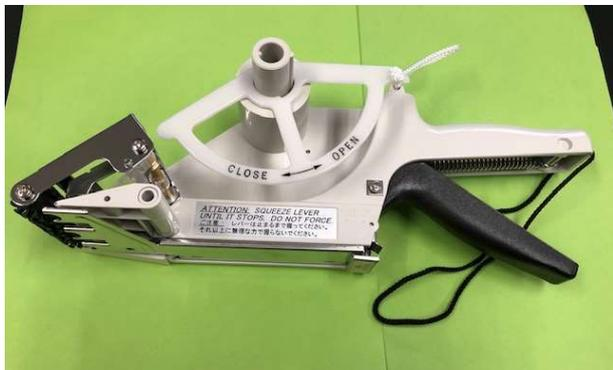
1. Turn the Label Holder counterclockwise to 'OPEN' and remove it.
