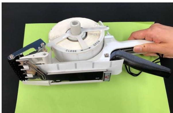
3. Lock it by pushing the Bottom Hook towards the opposite direction of a red arrow (OPEN).
