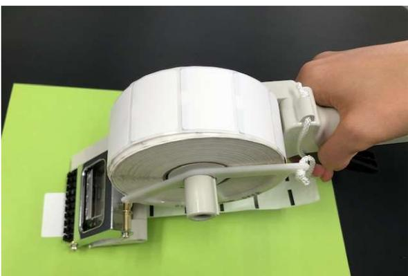
4. Stick a label on the object by squeezing a lever gently.
